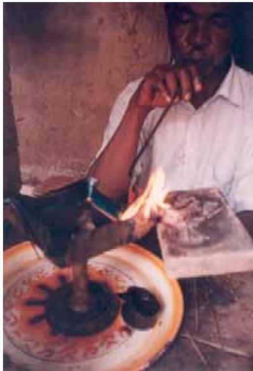
Fig. 2.2 Using the oil lamp and blowpipe to solder
