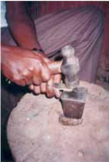
Fig 2.4 Hammering brass to make sheet metal
