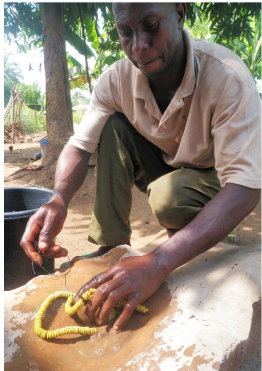
C. Global Mamas bead maker Moses removing powder and polishing the fired beads on sandstone with water.
