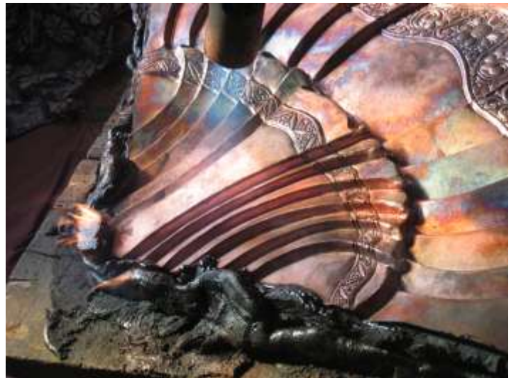
A piece of metal embedded in wax is annealed, showing the changes in color under the propane torch
