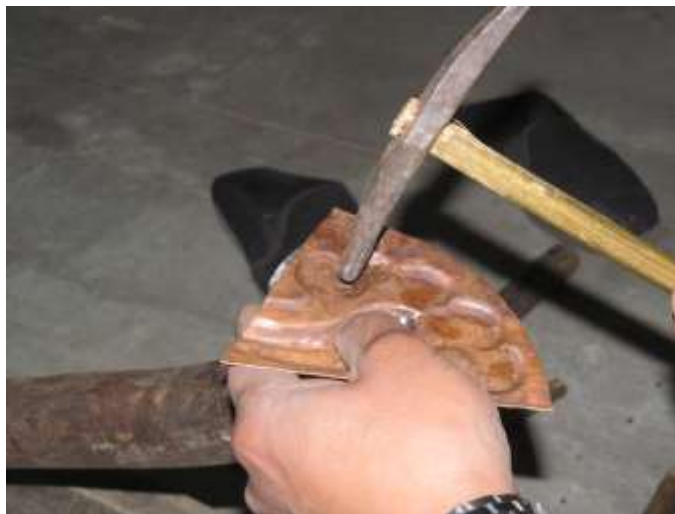
Embossing done from the back of a form
