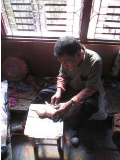
A worker sanding a finished piece to smooth and shine it
