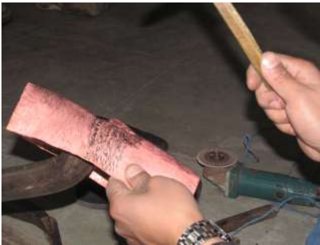
Embossing done from the front of a form
