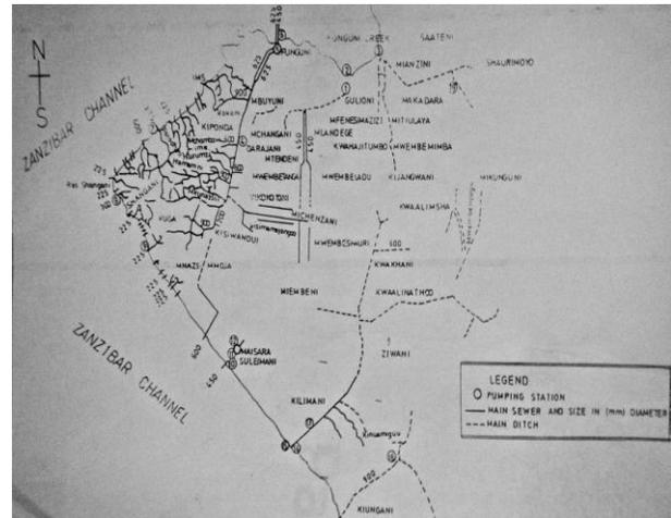
Figure 5. Stone Town runoff system. (Van Bruggen 1990.)
