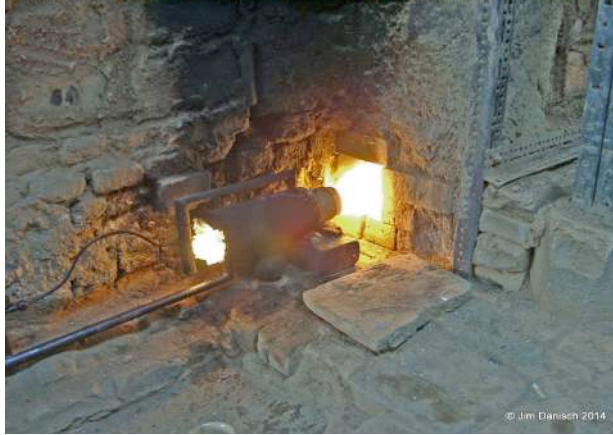
Figure 2: Danisch's kerosene burner at work
