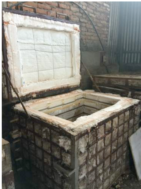
Figure 4: Kiln used at Everest Pottery for bisque and glaze firings
