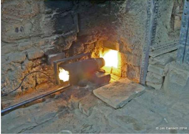
**Figure 2: Danisch's kerosene burner at work**
