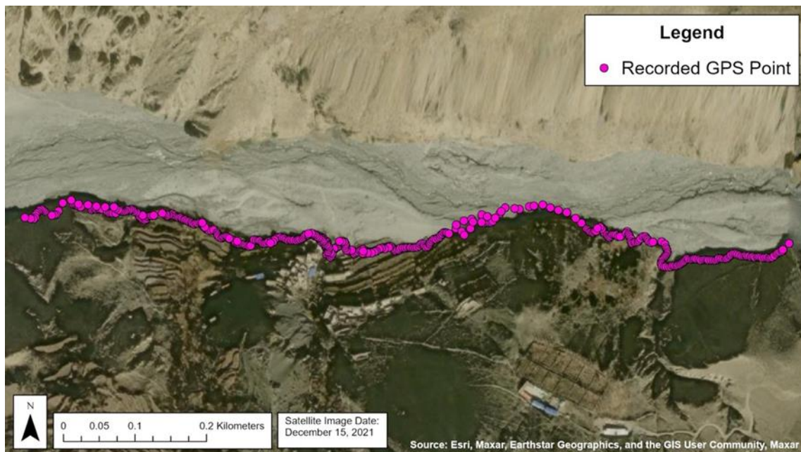
Figure 15: GPS Points Recorded while Walking the New Flood Line in 2022 and Plotted in ArcGIS Pro
