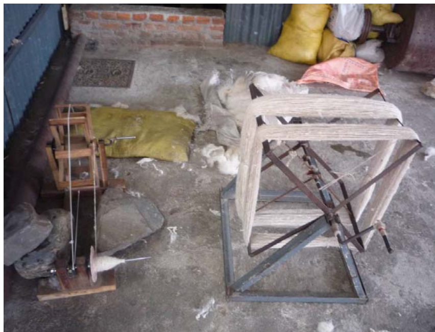
Below: The traditional Chakra used to spin wool into Yarn
