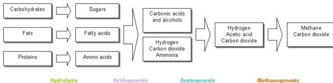
Anaerobic digestion occurs in three temperature ranges: psychrophilic (< 30°C), mesophilic (30-40 °C) and thermophilic (50-60 °C), with the highest rates of biogas production occurring in the mesophilic and thermophilic ranges (Yadvika et al., 2004). The pH of the digester is mainly affected by the production of carbon dioxide and volatile fatty acids; digestion occurs at a pH range of 5.5-8.5, however the optimal range is between 6.8 and 7.2 (Yadvika et al., 2004; Slater, 2007).
