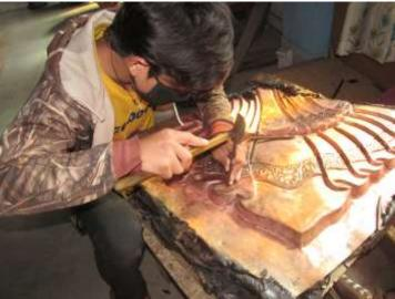
Member of the workshop carves a detail into a large piece of copper embedded in wax.
