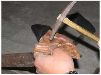
excess force. Working from the back side of the metal sheet the form is pounded out with heavy
