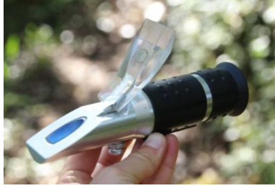
Figure D. Vee Gee BX-50 Refractometer. For determining sugar concentration in flower nectar.
