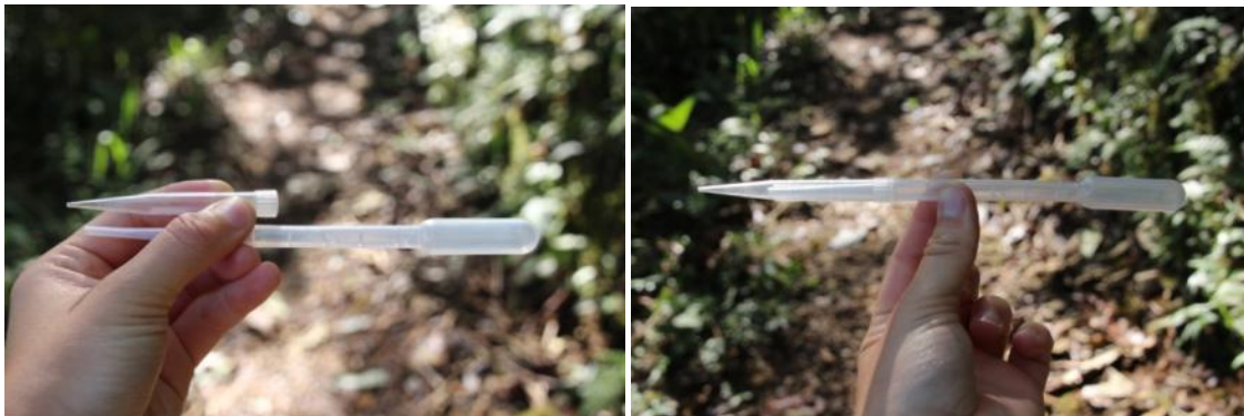
Figure E. Makeshift nectar extraction device: 3-mL plastic pipette with a VWR Ergonomic High-Performance 10-1000uL micropipette tip attached.
