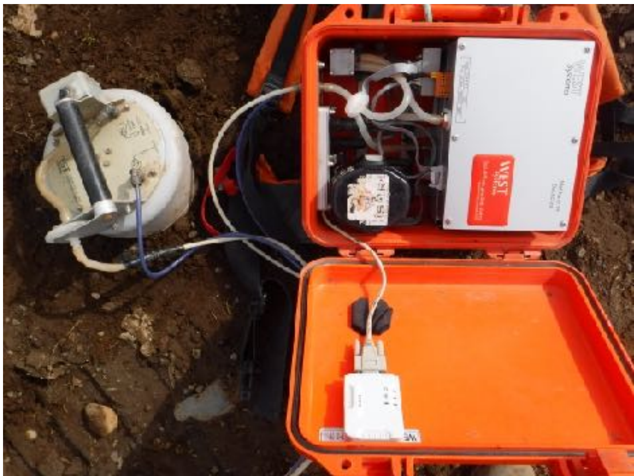
Figure 4. The West Systems 2012 static chamber fluxmeter. Gas collects in the circular chamber and is pumped through CH 4 and CO 2 IR detectors. Gas concentration data is transmitted wirelessly to a handheld computer.
