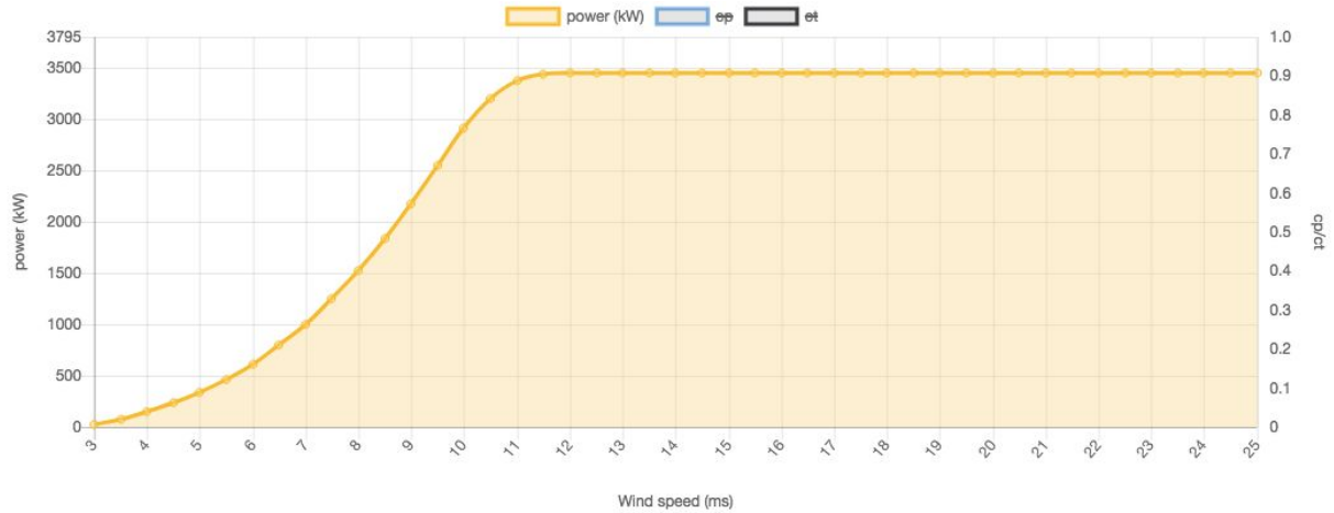
Figure 12. V117-3.45MW turbine power curve from wind-turbine-models.com. The V117-3.45 MW model cut-in wind speed is 3 m/s and cut-out speed is 25 m/s.
