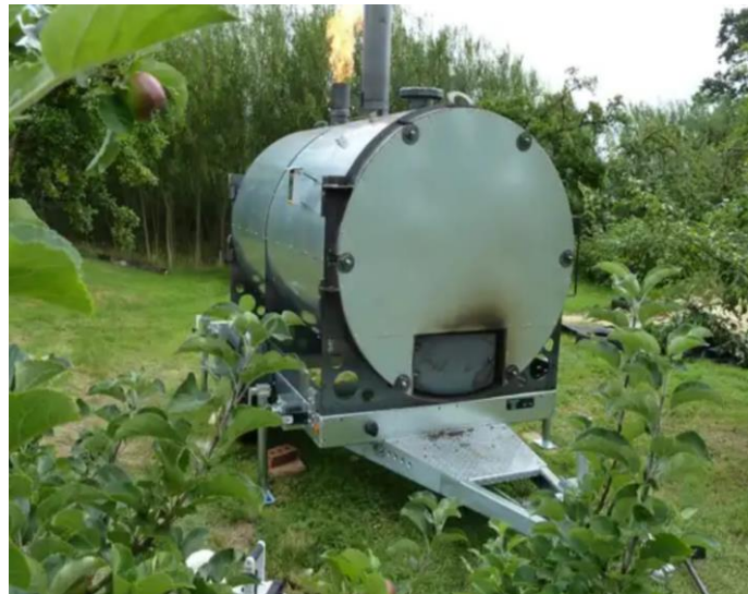
Figure 6: The Exeter Mobile Retort Kiln with a trailer attached. Retort Chamber Capacity – 1.7 cubic meters, approx. 500kg of fuelwood. Production cycle: 8-10 hours. Return per cycle: 170-195kg of charcoal. (online photo from Carbon Compost Company).
