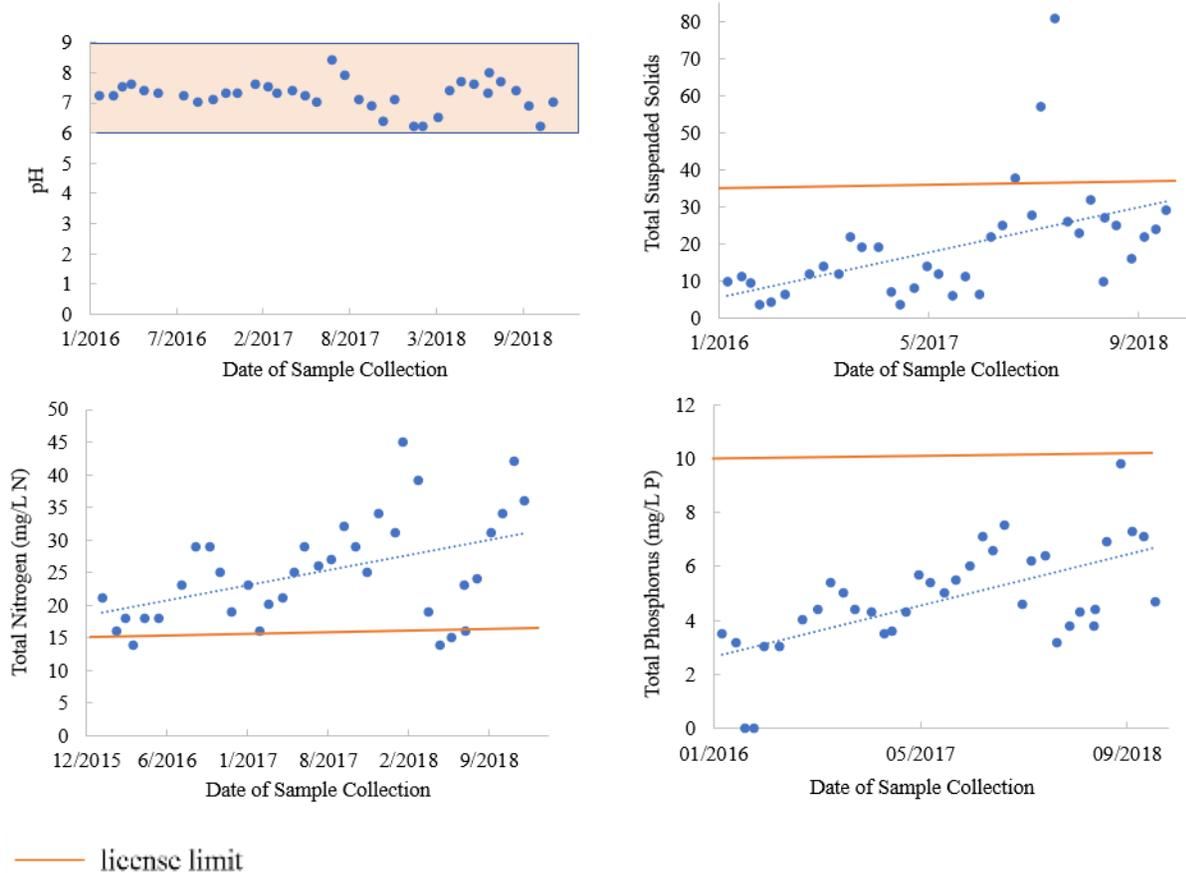
**Figure 4.** pH, total suspended solids, total nitrogen, and total phosphorus levels relative to license limits from 2016 to 2018
