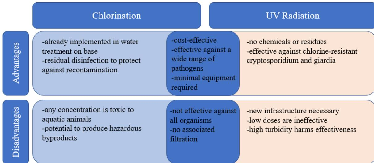
**Figure 7.** Comparison of the similarities and differences of chlorination and UV radiation
