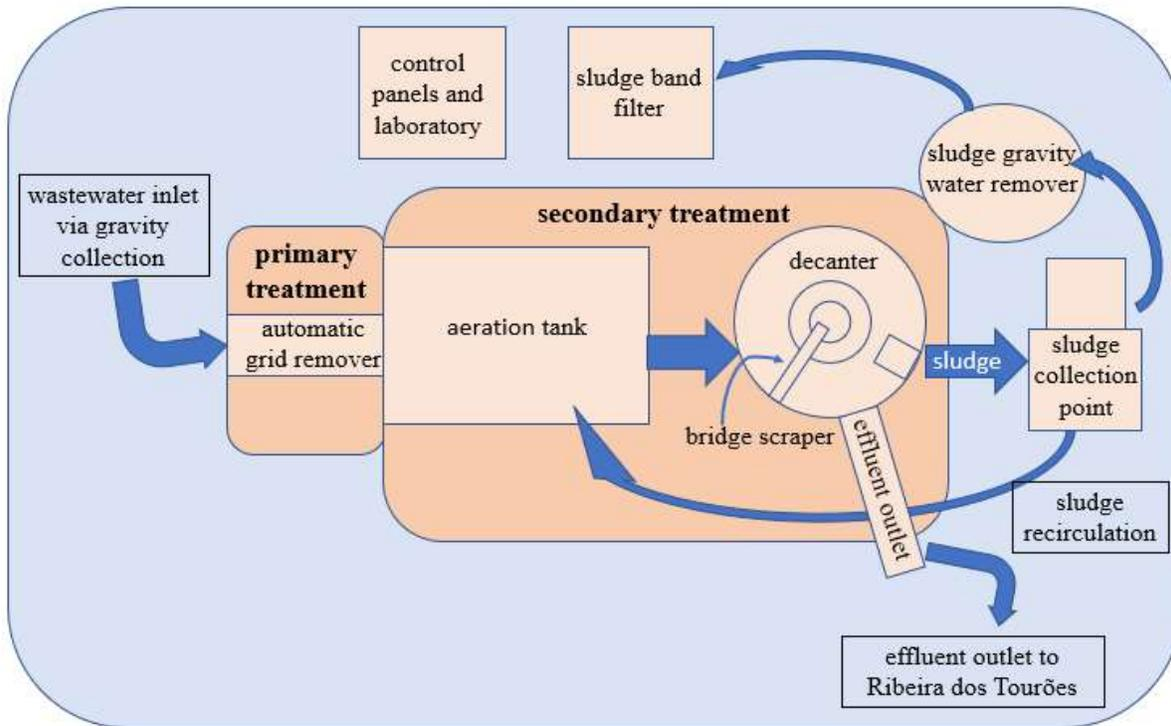
**Figure 1.** The flow of wastewater at the Base Aérea N.º5 wastewater treatment plant
