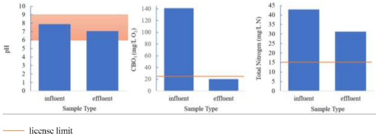
**Figure 3.** Influent and effluent pH, CBO<sub>5</sub>, and total nitrogen values relative to license limit
