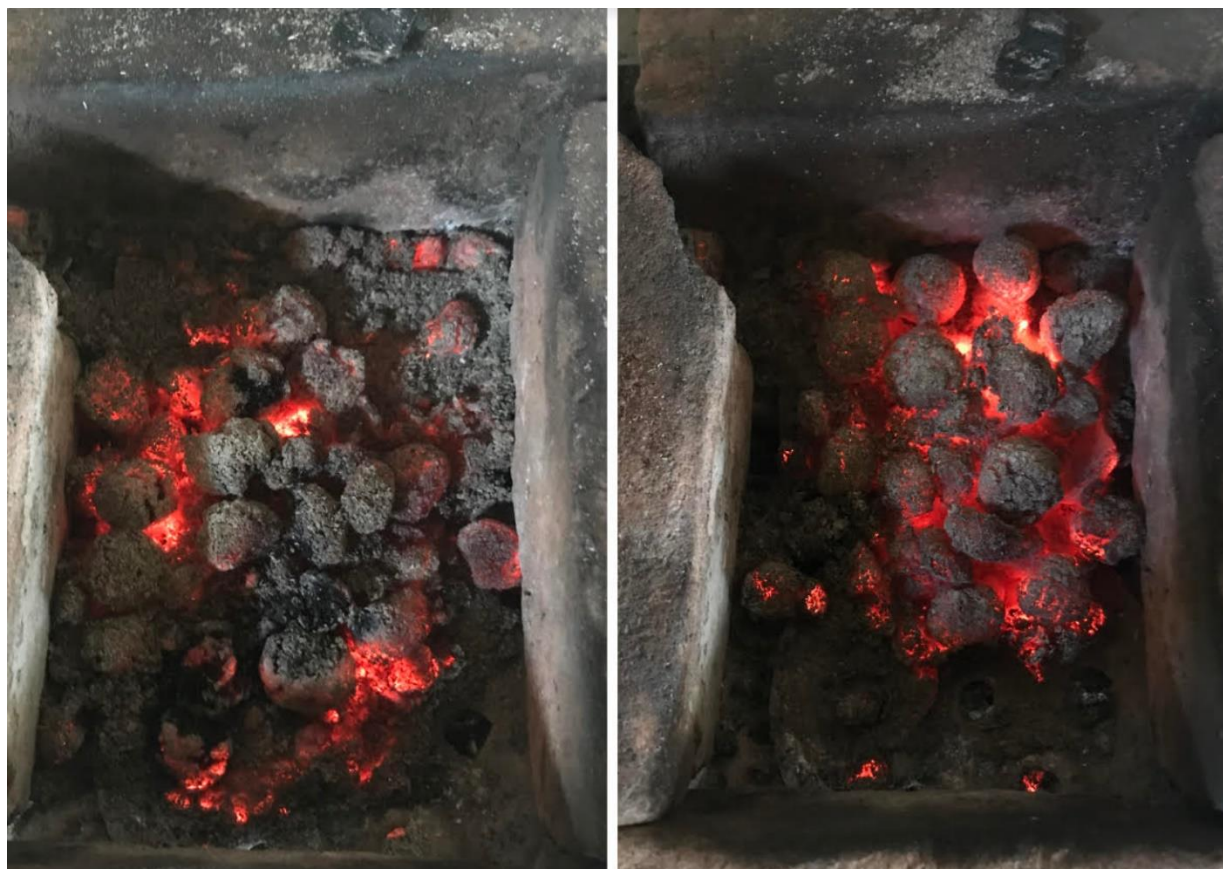
Figure 9: Cassava-based biofuel (left) and starch-based biofuel (right) after completion of Rice-Cooking Test. A large quantity of the cassava biofuel has turned to ash, whereas the starch biofuel can continue to be used for cooking.
