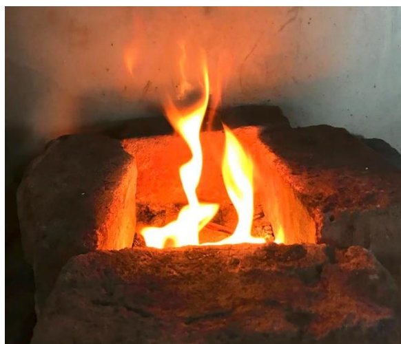
Figure 5: Clay stove used for Durability and Rice Cooking tests
