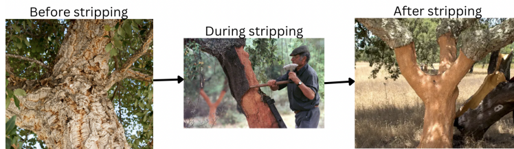
Figure 7. Cork extraction process
