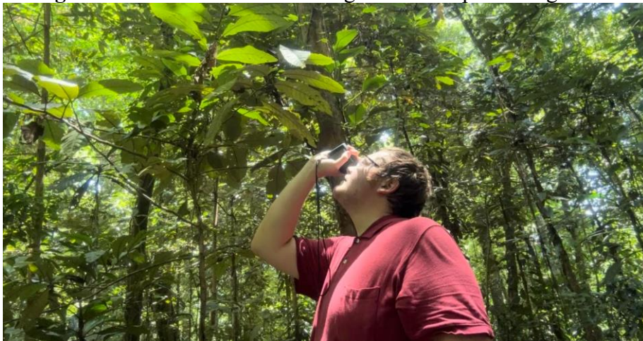
Figure 7. Tree height estimation using range finder in Drago Dos.
