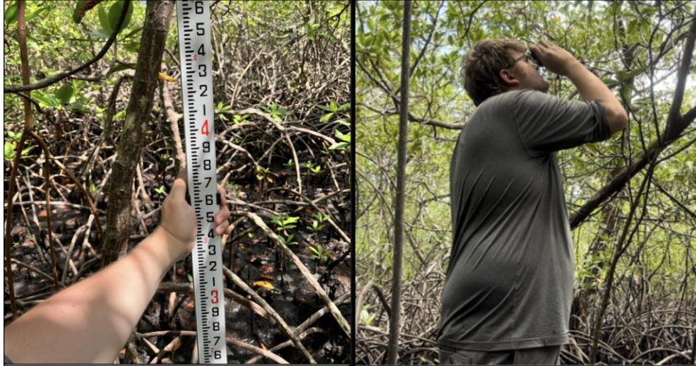
Figure 10. Tree height estimation using extendable measuring stick (left) and range finder (right) in mangrove forest.
